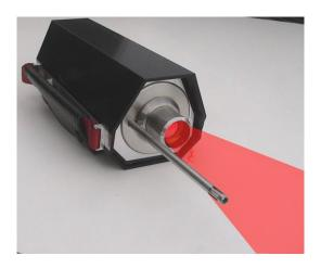
To focus an instrument that will be used in the field or out-of-doors, first set the instrument up in subdued lighting in a laboratory. There you will be able to see the light being emitted by the Light Emitting Diode (LED) and determine the distance to spot size ratio. Then, when you are in the field, you can determine the area being measured by knowing that the ratio of the distance to spot size will remain constant as it was in the lab.
